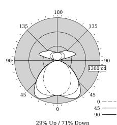
Total Output 4577 lm 99.5 lm/W Efficacy 3442K CCT CRI 82 R9 6 29% Up / 71% Down Distribution Spacing Criteria (0/90/180°) 1.14/1.61/NA
