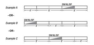
IMPORTANT: Whenever longer rows are made up of both 4' and 8' modules, EM/NL/BP sections will always be installed in 8' modules. If specific site restrictions require EM/NL/BP sections to be installed in 4' sections, please contact the factory.
