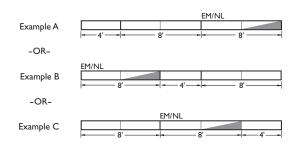
IMPORTANT: Whenever longer rows are made up of both 4' and 8' modules, EM/NL sections will always be installed in 8' modules. If specific site restrictions require EM/NL sections to be installed in 4' sections, please contact the factory.
