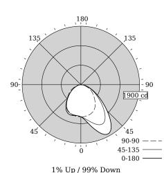
3216 lm Total Output 71.3 lm/W Efficacy ССТ 3494K CRI 84 R9 22 Distribution 1% Up / 99% Down Spacing Criteria (0/90/180°) 1.85/1.25/1.30
