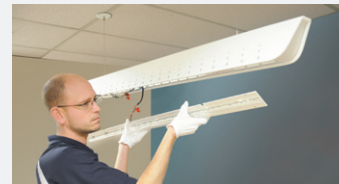
3. Remove the LED assembly.
