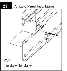
Secure variable panel to housing with screw provided.
