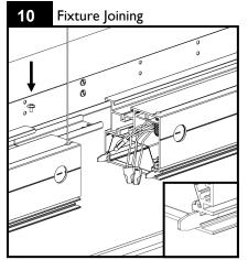
Secure joiner bracket to module I with screw provided. Slide module 2 on rail and engage on free end of joiner bracket. Complete all required electrical connections and tuck all wires inside both wiring cavities.
