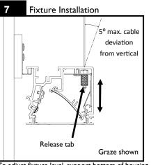
To adjust fixture level, support bottom of housing and release cable gripper by pulling tab as shown. Cable will slide freely and allow fine tuning of housing position. Repeat process at each cable gripper location using same procedure to ensure housing is level.
