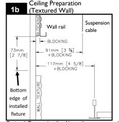
Optional: Textured walls. Above diagram covers all required dimensions for standard t-grid installation with a textured wall. <u>IMPORTANT:</u> To ensure a proper fit, blocking (by others) must be the same thickness as wall texture.
