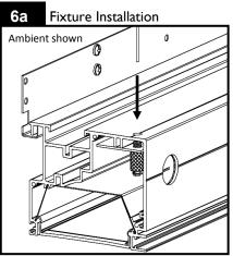
Insert suspension cables installed in step 3 through cable grippers inside fixture housing. <u>IMPORTANT:</u> Ensure suspension cables are vertical. Level fixture and trim excess cable to 1" below fixture. Tuck remaining cable inside fixture housing.
