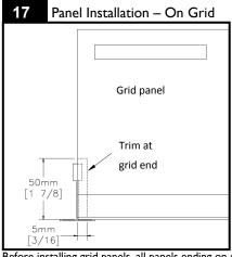
Before installing grid panels, all panels ending on grid must be trimmed as shown. Ensure one left and one right are trimmed for each required run.
