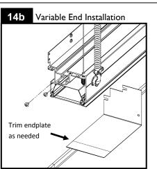
After fixture modules have been installed and levelled, measure distance between wall and fixture end. Trim variable endplate as required. <u>INSTALLATION</u> <u>TIP</u>: Before next step, attach 2 screws shown above to housing. Fully tighten then back off 1/2 turn.
