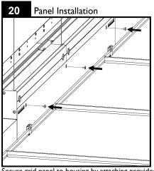
Secure grid panel to housing by attaching provided screws to housing through panel slots as shown. Repeat panel installation to complete run.
