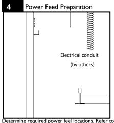
Determine required power feel locations. Refer to page I for typical power feed locations for each housing. Prepare power feed drop conduit and suspend close to required location. Attachment to fixture module is shown in step 8.
