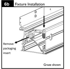
Engage housing on wall rail. Insert suspension cables installed in step 3 through cable grippers inside fixture housing. Pull cables through and refer to next step for levelling. <u>IMPORTANT</u>: Remove graze packaging insert from both ends of each housing.
