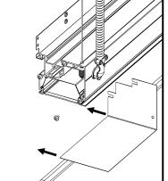
After variable endplate has been trimmed to size, slide endplate toward wall guiding open slots towards screws installed in step 14b. Hook slots on screws and push all the way towards wall.
