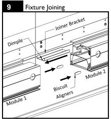
Slide dimpled side of joiner bracket approximately I inch inside top channel of module I. Tap biscuit aligners just past half way inside module 2 as shown.
