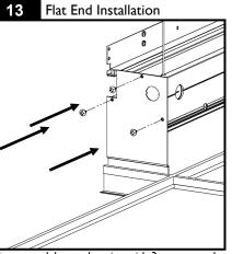
Secure endplate to housing with 3 screws as shown.
