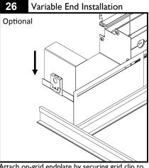
Attach on-grid endplate by securing grid clip to t-bar. Secure grid clip to t-bar following instructions shown in step 21.
