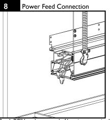
Break 7/8" knockout at end of housing at required power feed location. Install conduit connector (by others) and complete electrical connections. For a row end, tuck wires inside wiring cavity and follow endplate installation instructions starting in step 13.
