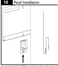
Insert grid clips (x2) to grid panel at slot locations. Push grid clip up as shown until bottom of clip is flush with bottom of grid panel.
