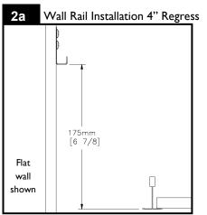
TruGroove perimeter fixture modules are available in two different above plenum heights. Refer to layout drawings for required regress. Standard 4" regress is shown in above diagram. Attach wall rails (hardware by others) to wall studs at specified height. <u>IMPORTANT</u>: Ensure all wall rails are level.
