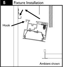
Lift fixture module past ceiling plane, Tilt as shown and engage housing hook on wall rail.
