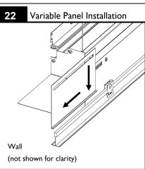
For variable ends at a wall, insert variable panel inside installed grid panel. Slide to required position. <u>NOTE</u>: When installed, the variable panel will match the length of variable endplate installed in steps 14b-16.
