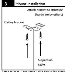
Refer to page I and steps Ia/Ib above for determining mounting locations. To install the 1st module, two brackets and suspension cables are required. When joining luminaires, only one bracket and suspension cable are required for each joining module.
