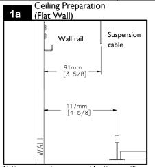
Ceiling preparation covers grid ceiling modifications, attachment of wall rails and mount installation. Above diagram covers all required dimensions for standard t-grid installation. <u>IMPORTANT</u>: Grid opening size must be followed for proper fit.
