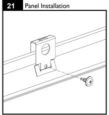
Secure grid clips to t-bar ceiling using screws (by others).
