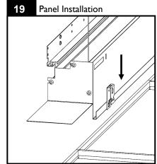
Starting at one end, align first grid panel with end of housing and slide onto t-grid to engage clips.
