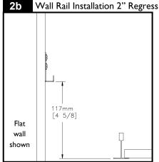
Optional 2" regress is shown in above diagram. Attach wall rails (hardware by others) to wall studs at specified height. <u>IMPORTANT</u>: Ensure all wall rails are level.
