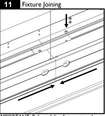
IMPORTANT: Before sliding fixtures together, make sure all electrical wires and suspension cables are properly tucked inside fixture wiring cavities. Slide fixture housings together and attach second joiner bracket screw.
