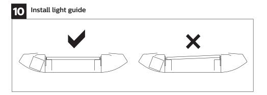
**Identify smooth side of the Light Guide and ensure it is installed smooth side DOWN**. Install Light Guide panel into LED fixture after joining and wiring is complete. Ensure panel is seated correctly as shown above.
