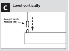
LEVEL VERTICALLY (shown above): Support fixture from below and use supplied aircraft cable release tool to make fine height adjustments (see instruction A for details).
