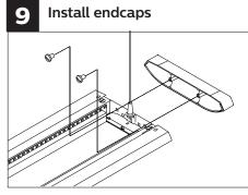
Attach end caps using supplied #8 screws.
