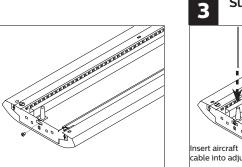
With 2 people, raise the first fixture to the ceiling. At each end of the module, insert aircraft cable through aircraft cable adjuster (located on A/C mount bracket). The adjuster will automatically grip and hold the cable. IMPORTANT: Do not force cable into adjuster. See instruction A (next page) for details. Trim aircraft cable below adjuster as per instruction A (next page).
