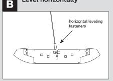
LEVEL HORIZONTALLY (shown above): Loosen fasteners on bottom of adjuster and level as required. Tighten fastener once fixture is in level position.
