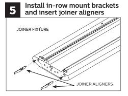
For each additional fixture in the row, at the end furthest from the existing suspended fixture, attach A/C mounting bracket to fixture using supplied fasteners (see step 2). At the end closest to the existing suspended fixture, insert joiner aligners into crossplate (aligners will lock into place).
