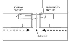
With two people, raise second fixture to ceiling. At joint, insert joiner aligners through black gasket and into suspended fixture. At other end (opposite joint), insert aircraft cable through adjuster.
