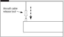
LEVEL VERTICALLY (shown above): Support fixture from below and use supplied aircraft cable release tool to make fine height adjustments (see instruction A for details).
