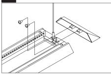
Attach end caps using supplied #8 screws.
