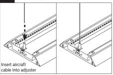
With 2 people, raise the first fixture to the ceiling. At each end of the module, insert aircraft cable through aircraft cable adjuster (located on A/C mount bracket). The adjuster will automatically grip and hold the cable. IMPORTANT: Do not force cable into adjuster. See instruction A (next page) for details. Trim aircraft cable below adjuster as per instruction A (next page).
