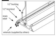
NON-POWER LOCATIONS: Cap all wires and tuck into wire cavity.
