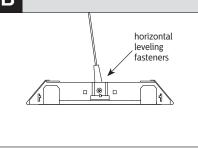
LEVEL HORIZONTALLY (shown above): Loosen fasteners on bottom of adjuster and level as required. Tighten fastener once fixture is in level position.
