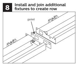
With two people, raise second fixture and engage on mounting brackets (see STEP 4). At joint, remember to insert black gasket.
