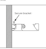
With 2 people, raise fixture into position and engage it on hooks located on top of wall brackets, then rotate it down into position. Secure bracket using supplied hardware.
