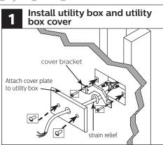
Determine power feed location and install 2"x4" utility box (supplied by others) parallel with fixture. Complete connections at utility box with supplied power cord. Attach cover bracket using supplied hardware. Punch power access hole in supplied cover, feed power cord through and attach strain relief on wall side. Attach cover using supplied painted hardware.
