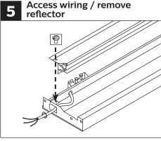
To access wiring, remove screw from top reflector and lift reflector off.
