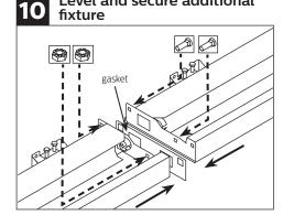
Level second fixture by adjusting the tilt screw (see step 7). Slide second fixture flush against first fixture and secure joint using supplied nut and bolt hardware (requires 3/8" nut drivers). Secure fixture to wall brackets by tightening the lock screw at each bracket location (see step 7).
