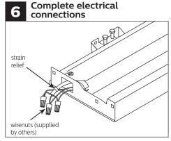
Complete electrical connections using wire nuts (supplied by others). Re-install reflector and hardware removed in STEP 5.
