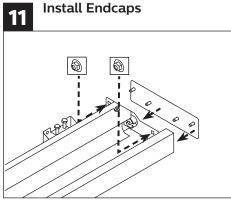
Attach endcap to first and last module in each row using supplied hardware.
