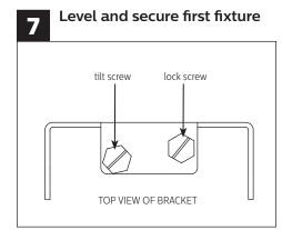
LEVEL: Using 5/16" hex nut driver, level fixture by adjusting the tilt screw.
