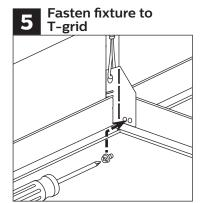
Use a #8x1/4" sheet metal screw to fasten fixture to T-grid and use a hanger wire to tie off appropriately in accordance with local building codes (screws and hanger wires supplied by others).
