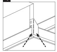
Bend tabs flush against T-grid in order to clear corner for ceiling tile.
