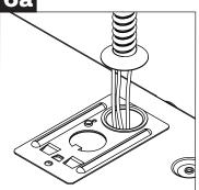
Optional Flex whip is prewired inside fixture. Remove packaging and insert snap-in fitting into wiring cover. Complete electrical connections at other end of whip in accordance with local building codes.
