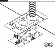
Make all electrical connections to the fixture.
