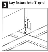
Lay fixture into T-grid.
