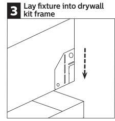
Lay fixture into drywall kit frame.
