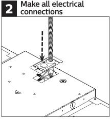
Make all electrical connections to the fixture. Attach wire access cover plate.
