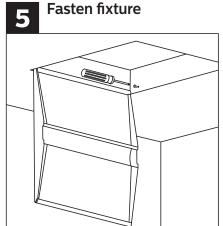
Use a #8x1/4" sheet metal screw (supplied by others) to fasten fixture to drywall kit frame from inside of housing. Repeat on each corner.
