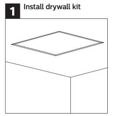
Install drywall kit frame in ceiling. Refer to Drywall Kit specification sheet for mounting options and ceiling opening sizes.
