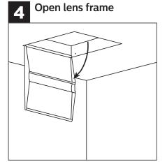
Push up on center channel of lens frame and shift in direction of hinges. Lens frame will then swing open in a downward direction. If fixture has lens frame restraint, release by pressing inwards.
