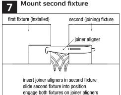
Insert joiner aligners into second (joining) fixture. Raise second fixture into position; at end opposite joint, engage fixture into wall mount bracket (shown in STEP 5). At joint, carefully slide fixture into position so that first and second fixtures are engaged on joiner aligners.
