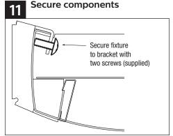
Secure fixture(s) to wall mount brackets with two screws (supplied,  $\#10-32 \times 1/2"$ ) at each bracket location.
