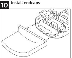
Install endcaps using supplied hardware. NOTE: Two different endcaps supplied (left/right).
