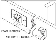
Install additional wall mount brackets as required for single fixture or continuous rows. Ensure additional brackets are level with first bracket.
