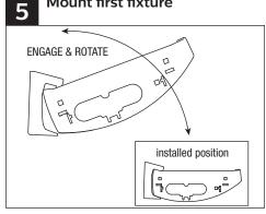
Raise first fixture into position and engage it on wall brackets, then rotate it down into position (as shown).
