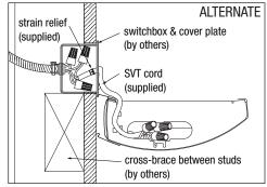
RECOMMENDED: For best mounting aesthetics, install switchbox flush with finished wall directly behind fixture's specified power location. Install two studs at mounting location. Leave enough gap between studs to accommodate standard switchbox mounted sideways (about 4"). Make electrical connections in switchbox with supplied SVT cord. Secure power cord with supplied strain relief on the switchbox side.
