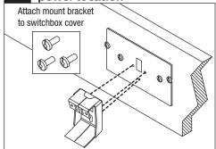
RECOMMENDED: Attach wall mount bracket to switchbox cover plate with 3 screws (supplied). Leave power cord outside wall for connection.
