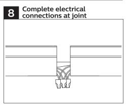
Complete electrical connections at joint using supplied quick-wire connectors. Tuck wires into wiring cavity.
