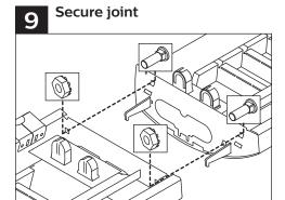
Secure joint using suppllied nuts and bolts. Ensure star washer side faces against metal plate at end of feeture.
