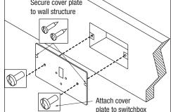
Feed SVT cord through hole in supplied switchbox cover plate. Attach cover plate to switchbox with two screws (supplied by others). Secure cover plate to wall structure with two structural screws (supplied by others)
