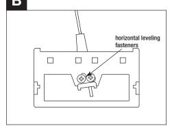
**LEVEL HORIZONTALLY** (shown above): Loosen fasteners on bottom of adjuster and level as required. Tighten fastener once mount is in level position.
