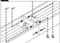
**SLIDE MODULES TOGETHER:** Secure joint from above using supplied nut and bolt hardware.
