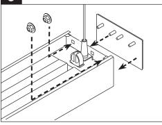
Attach endcap to first and last module in each row using supplied hardware. Attach nuts to 2 outer endplate studs.
