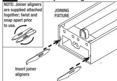
For each additional fixture in the row, at the end furthest from the existing suspended fixture, remove required rectangular knockout(s) in socket saddle and drop A/C mounting bracket through the top. Attach A/C mounting bracket to fixture using supplied fasteners (see step 2). At the end closest to the existing suspended fixture, insert joiner aligners into crossplate (aligners will lock into place).
