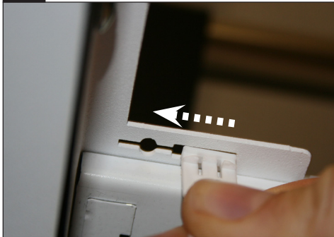
While supporting from below, insert loose end of retention strap into rectangle end of slot and slide towards end of the fixture until it clicks into position. Repeat at opposite end.
