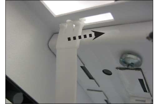
While supporting the doorframe from below, detach the retention strap from the housing (at fixture end) by sliding sideways towards the center of the fixture and pulling out of the slot. Repeat at opposite end of fixture.
