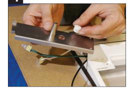
Snap bushing (power locations) or plug (non-power locations) into in-run mount bracket (image shows in-run bracket with plug for non-power location). With tabs on bracket facing outward, slide bracket into joint end of fixture. Attach bracket using supplied hardware.
