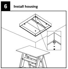
Attach housing to anchors using 1/4'-20 hex nut and washer (supplied by others)
