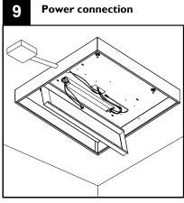
Complete electrical connections and reinstall wire cover
