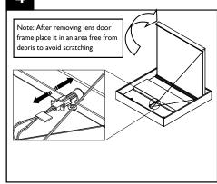
Pull the lens door frame upward on the indicating marker side. Disconnect wire harness and remove doorframe.
