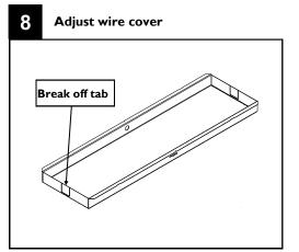
On the conduit entry side of wire cover break off tab to allow conduit to enter driver channel
