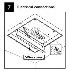
Remove wire cover from housing. Make all necessary power connections and reinstall wire cover.
