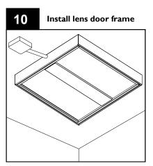
Connect and re-install lens door frame. Align door frame so that it sits flush with the bottom of the housing.
