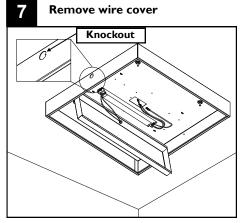
Remove wire cover. Push in knockout on the side of housing for conduit entry.
