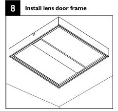
Connect and re-install lens door frame. Align door frame so that it sits flush with the bottom of the housing.
