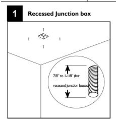
Use installation dimensions supplied on page 3, to mark up and drill holes in the correct locations. Install 1/4"-20 anchors (supplied by others) to ceiling making sure they protrude between 7/8" to 1-1/8" and that the wire access hole is over the junction box.
