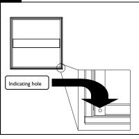
Locate indicating holes on lens door frame. These markers are opposite to the doors hinging mechanism.
