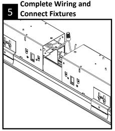
Install the joiner fixture into the T-Bar Grid from above. Complete wiring and slide the fixtures together.
