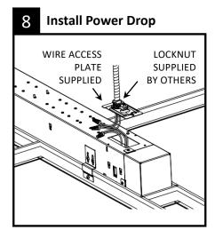
Install power drop at desired location. At the power location(s), remove factory installed wire cover. Feed power wires through. Complete all wiring connections.
