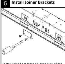
Install joiner brackets on each side of the housing using supplied hardware.
