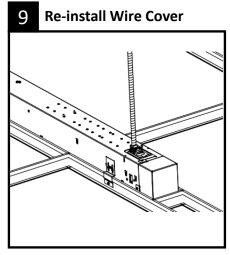
Re-install wire cover and slide to lock. Install screw.
