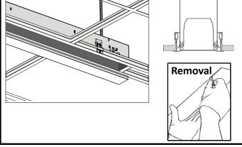
Flush Lens: Snap in lens into fixture.
