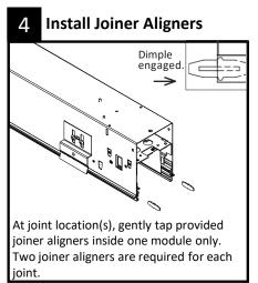
Important: To insert aligners, tap gently with a hammer until half is inserted into the joiner channel. Be sure to engage the dimple.
