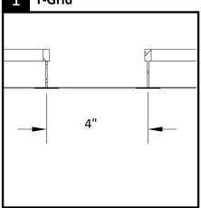
Install main T's, 4" on center. For continuous row lengths, refer to supplied layout drawings. Add 1/4" to the overall housing length indicated on your layout drawings. Position the cross T.
