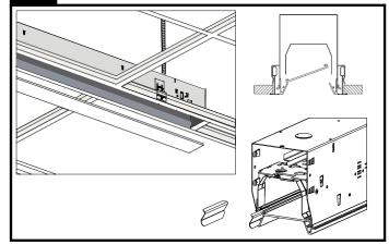
**Regressed Lens:** Angle lens to insert into fixture. Lay lens on aluminum extrusion flange.
