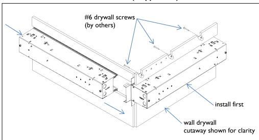
Inside corner kit for wall-to-wall configuration requires the installation of the locking endplate fixture as a first step. Insert fixture inside wall making sure a 4" to 1/2" overlap exists inside wall. If fixture needs to be joined to other fixture, follow steps 2 and 3 on page 8. Level fixture and secure to drywall using #6 drywall screws (by others). IMPORTANT: Attach screws through large holes in aluminum trim every 9 inches on both sides of fixture housing.
