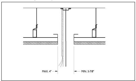
Install 'C' channel along full fixture perimeter to cutout specified drywall and cut opening to dimensions shown.
