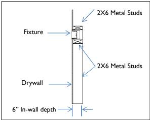
Wall construction requires the use of 2X6metal studs (or equivalent) and a minimum in-wall depth of 6".
