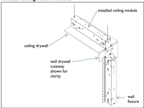
After all ceiling fixtures have been fully installed, secure to drywall using #6 drywall screws (by others). IMPORTANT: Attach screws through large holes in aluminum trim every 9 inches on both sides of fixture housing.
