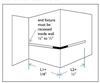
Wall cutout dimensions for outside corners are based on dimensions provided on layout drawings.
