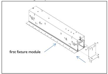
Install locking endplate with supplied hardware to fixture module fixture module to be installed in ceiling. If power connection is not required at this end, cap wires and access plate prior to endplate installation.
