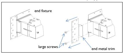
Installation of an end fixture at a wall end does not required the use of an inside corner kit. Prior to installation of this fixture module, remove factory installed metal end trim and 2 large head screws as shown in step 6.
