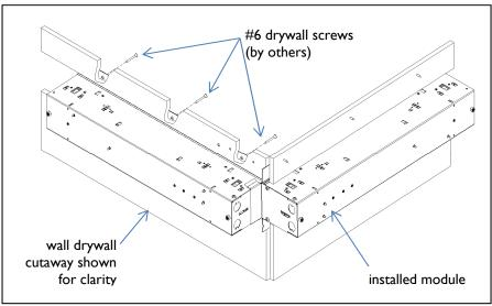
Insert joining module inside wall and slide towards installed module. Push joining fixture against installed fixture and secure to drywall with #6 drywall screws (by others). IMPORTANT: Attach screws through large holes in aluminum trim every 9 inches on both sides of fixture housing.
