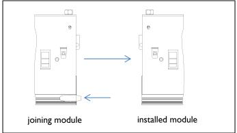
**Installation Tip:** For easier installation in cases where last fixture module ends at inside wall or end, tap aligners inside fixture modules together and secure with drywall screws. trim so that only 1/8" is visible before joining and attaching module.
