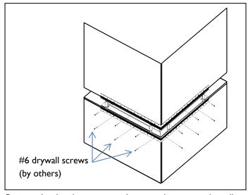
Position, level and secure outside corner housing to drywall with #6 drywall screws (by others) spaced 9" apart.
