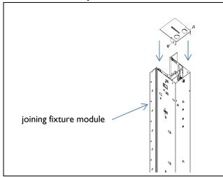
Install flat endplate with supplied hardware to fixture module to be installed in wall. If power connection is not required at this location, cap wires and access plate prior to endplate installation.
