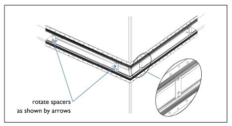
After securing fixture with drywall screws every 9 inches, remove internal spacers by rotating in direction shown by arrows.
