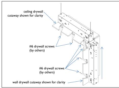
Raise first wall fixture to ceiling and engage housing body inside locking endplate in ceiling fixture. Push vertical fixture against ceiling fixture and secure to drywall with #6 drywall screws (by others). IMPORTANT: Attach screws through large holes in aluminum trim every 9 inches on both side of fixture housing.
