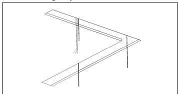
After drywall is installed, check that fixture opening is straight and that it meets required dimensions of minimum 3-7/8" to maximum 4".
