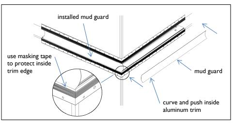
Install supplied mud guards inside each fixture. At corners, overlap and trim as needed to ensure a tight seal. **IMPORTANT:** To prevent debris from entering fixture, apply masking tape to inside edges of fixture trim, on both sides and full length of fixture run.
