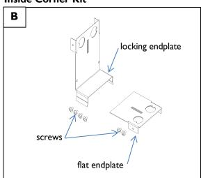
Inside corner kit parts: locking endplate, flat endplate,
