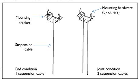
Install mounting brackets, suspension cables and power cables at required locations. Use one bracket and one suspension cable at end condition. Use one bracket and 2 suspension cables at a joint condition. Mounting bracket must be centered above fixture joint. NOTE: Mounting hardware by others.
