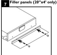
Attach filler panels to ends of housing using two supplied screws shown above.
