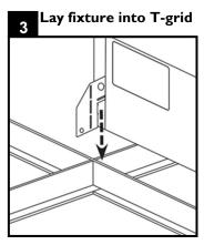
Lay fixture into T-grid.
