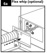
Optional Flex whip is prewired inside fixture. Remove packaging and insert snap-in fitting into wiring cover. Complete electrical connections at other end of whip in accordance with local building codes.
