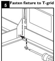
Use a #8x1/4" sheet metal screw to fasten fixture to T-grid and use a hanger wire to tie off appropriately in accordance with the local building codes (screws and hanger wires supplied by others.
