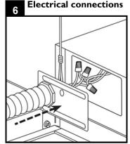
Make all electrical connections to the fixture.
