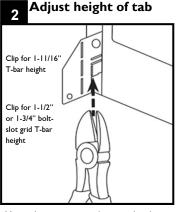
Use side cutters to adjust each tab to height of T-grid.
