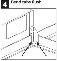
Bend tabs flush against T-grid in order to clear corner for ceiling tile.
