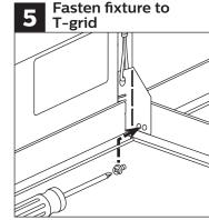
Use a #8x1/4" sheet metal screw to fasten fixture to T-grid and use a hanger wire to tie off appropriately in accordance with local building codes (screws and hanger wires supplied by others).
