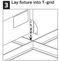
Lay fixture into T-grid.
