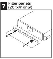
Attach filler panels to ends of housings using two supplied screws shown above.
