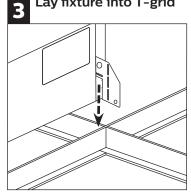
Lay fixture into T-grid.
