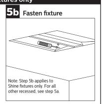
Use a #8x1/4" sheet metal screw (supplied by others) to fasten fixture to drywall kit frame from inside of housing. Repeat on each corner of exposed side, then move lens back into position and repeat Steps 4b and 5b on other side.
