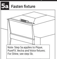
Use a #8x1/4" sheet metal screw (supplied by others) to fasten fixture to drywall kit frame from inside of housing. Repeat on each corner.
