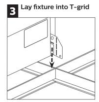
Lay fixture into T-grid.
