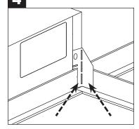
Bend tabs flush against T-grid in order to clear corner for ceiling tile.
