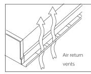
The air return version features slotted vents along the sides of the fixture. As a result, the installation method of the air return version is different to the standard version, and the fixture cannot be installed in continuous rows.
