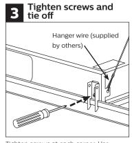
Tighten screws at each corner. Use hanger wire (supplied by others) to tie off appropriately in accordance with local building codes.
