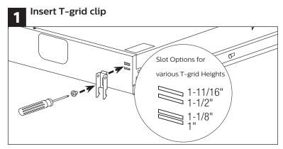
Insert T-grid clip (supplied) into correct slot to accomodate T-grid height. Hold in place with screw (supplied), but do not fully tighten screw until Step 3. Repeat at each corner of the fixture.
