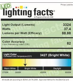
All results are according to IESNA LN-79-2008: Approved Method for the Electrical and Photometric Testing of Solid-State Lighting. The U.S. Department of Energy (DOE) verifies product test data and results.
