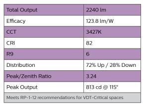
Photometry based on 4ft white luminaire. Black, Titanium and Custom color finishes may reduce delivered lumens. Custom color finishes may shift output color temperature.
