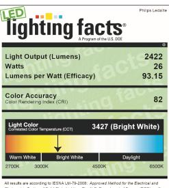
All results are according to IESNA LM-79-2008: Approved Method for the Electrical and Photometric Testing of Solid-State Lighting. The U.S. Department of Energy (DOE) verifies product lest data and results.
