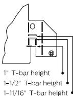
Integrated mounting tabs can be field-adjusted to various T-Grid ceiling heights for fastening directly to the T-Bar and/or tied off to the building structure.
